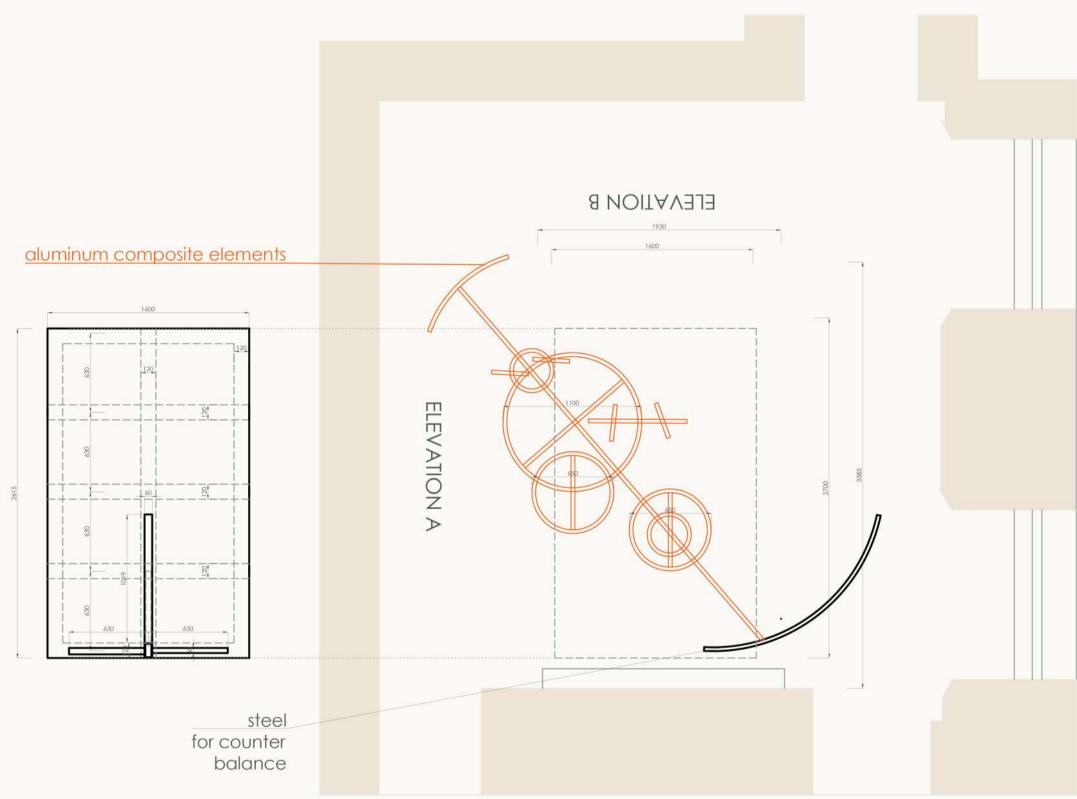
isolated plan view of subframe and aluminium composite elements scale 1:30
